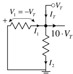
$I_T = 10V_T + V_T / R_1 + V_T / R_2 \approx 10V_T \Rightarrow R_I = V_T / I_T = 1 / 10 = 0.1\Omega$
